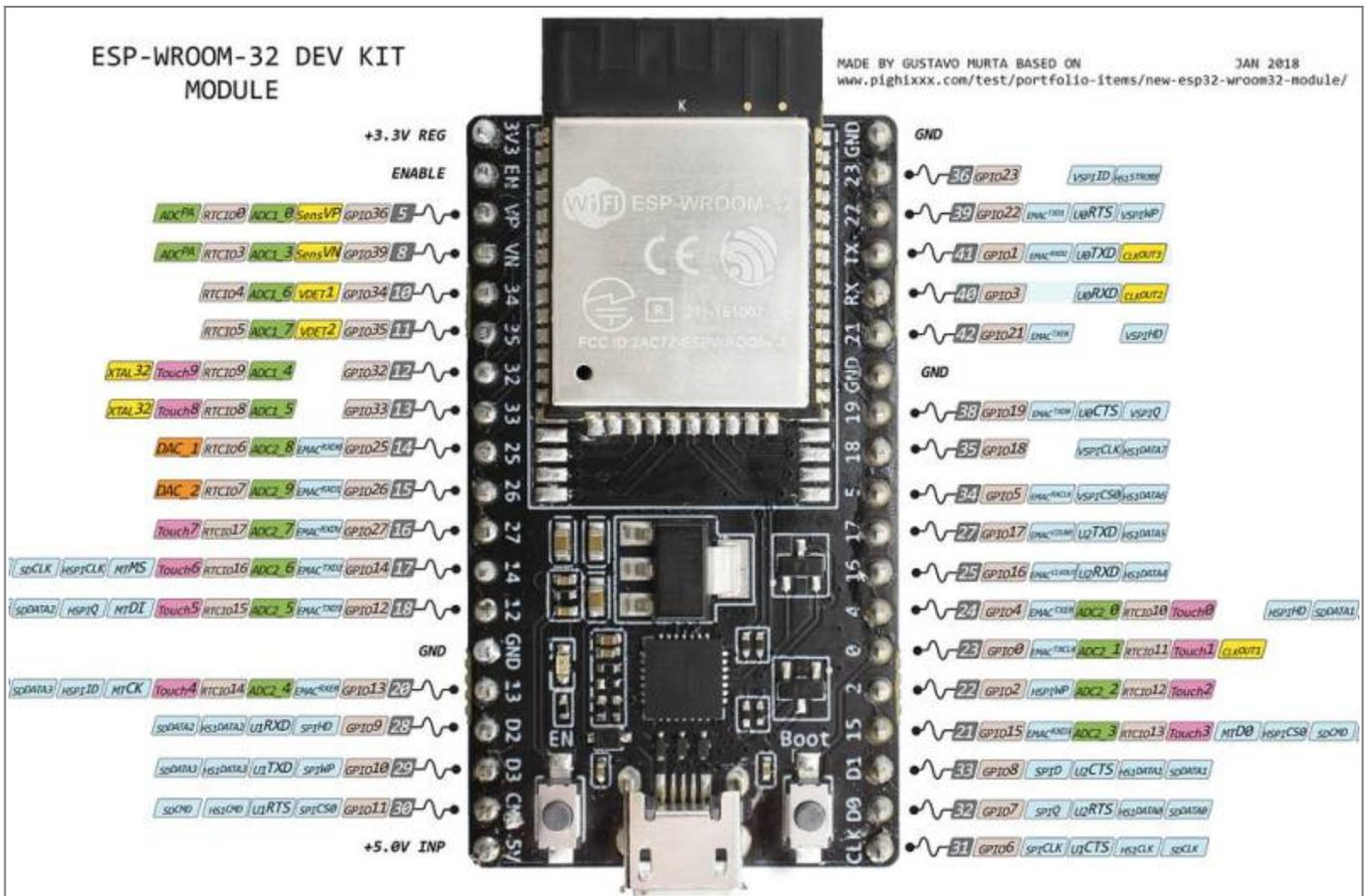
**Figure 1** ESP32 DevKit Pinout (Source: [ESP32 DevKit 38 Pins](#))
