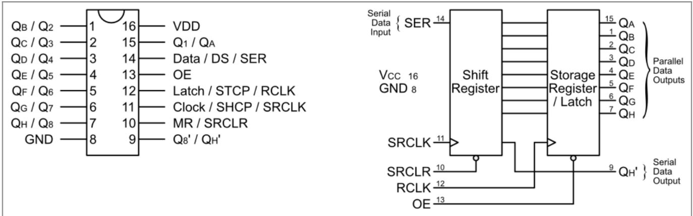
**Figure 2** SN74HC595(N) pinout diagram (left) and logic diagram (right), there are different names and abbreviations for the pins depending on the source; the labels in the logic diagram are the official ones from the datasheet (also see table 2).
