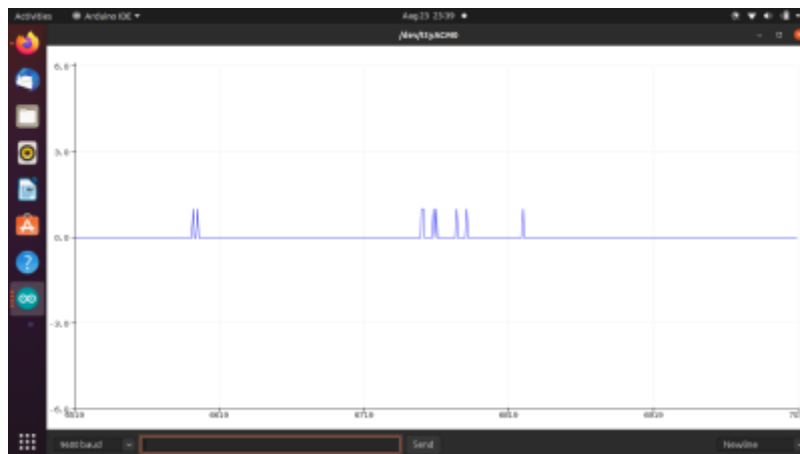
Figure 7 : Serial Plotter: Adjustment of the sensor sensitivity using the potentiometer
