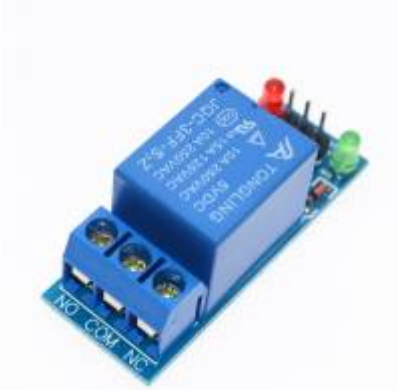
Figure: Relay module, https://www.stephenwenceslao.com/sites/default/files/1-relay-module4.jpg
