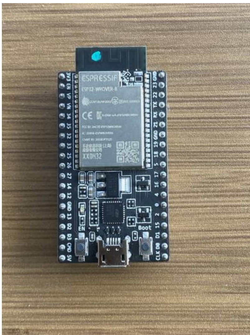
Fig.1: The ESP32 WROVER-B MODULE
