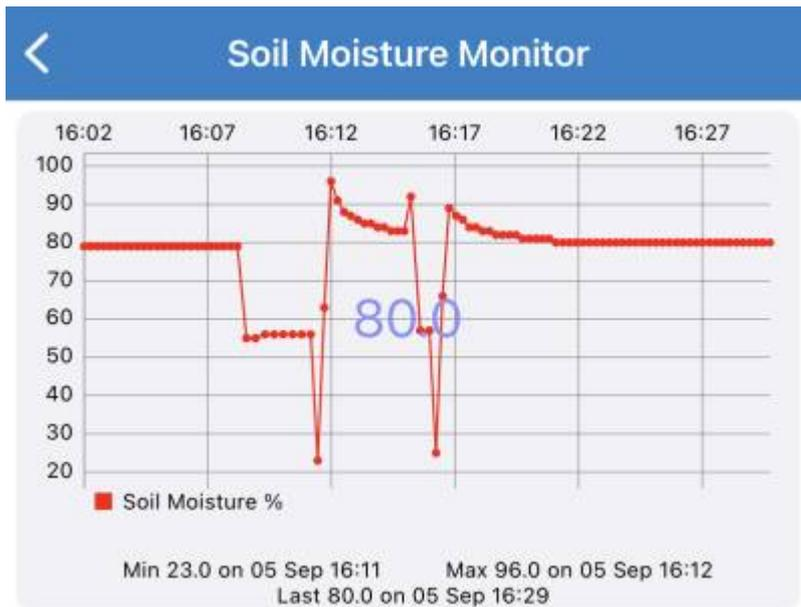
Fig.6 Shows a graphs of the soil moisture percentage obtained directly from ThingSpeak live stream data channel
