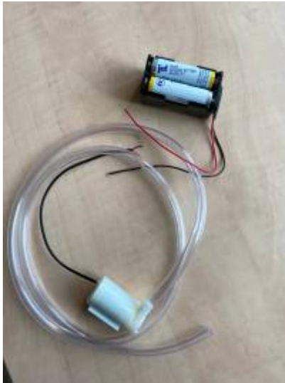
Figure 5.0 Water pump and battery pack
