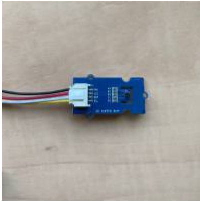
Figure 3.0 Grove Temperature and Humidity Sensor(SHT31)
