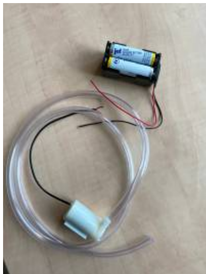
Figure 5.0 Water pump and battery pack
