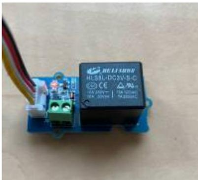
**Figure 6.0** Relay Module
