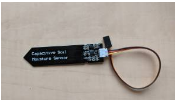
Figure 4.0 Capacitive Soil Moisture Sensor
