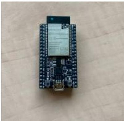
**Figure 2.0** Espressif ESP32 DevKitC
