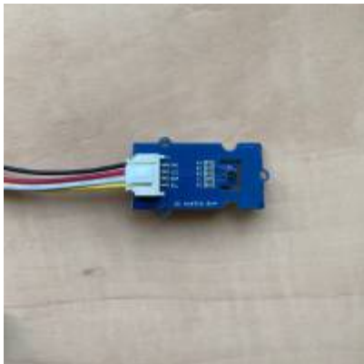
Figure 3.0 Grove Temperature and Humidity Sensor(SHT31)
