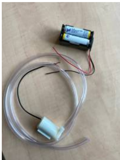
Figure 5.0 Water pump and battery pack
