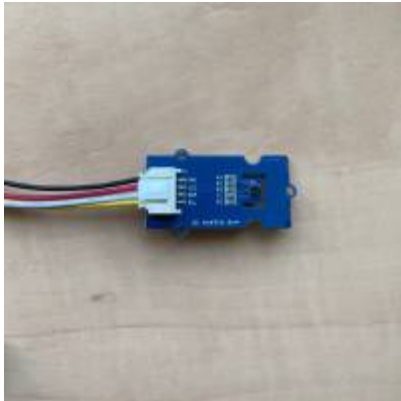
Figure 3.0 Grove Temperature and Humidity Sensor(SHT31)
