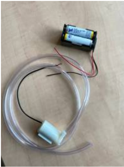
Figure 5.0 Water pump and battery pack
