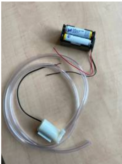
Figure 5.0 Water pump and battery pack
