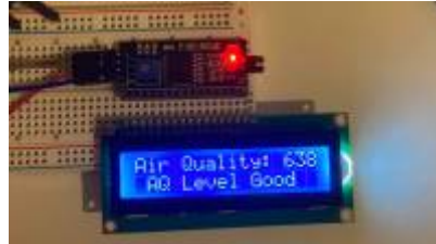
Figure 4: Liquid Crystal Display (LCD) screen (16 x 2) paired with I2C
