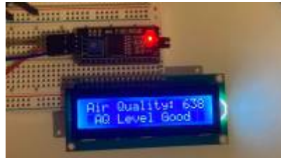
Figure 4: Liquid Crystal Display (LCD) screen (16 x 2) paired with I2C
