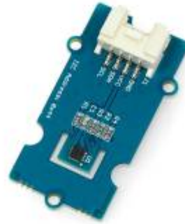
Figure 6 SHT31 Temperature and Humidity Sensor.
