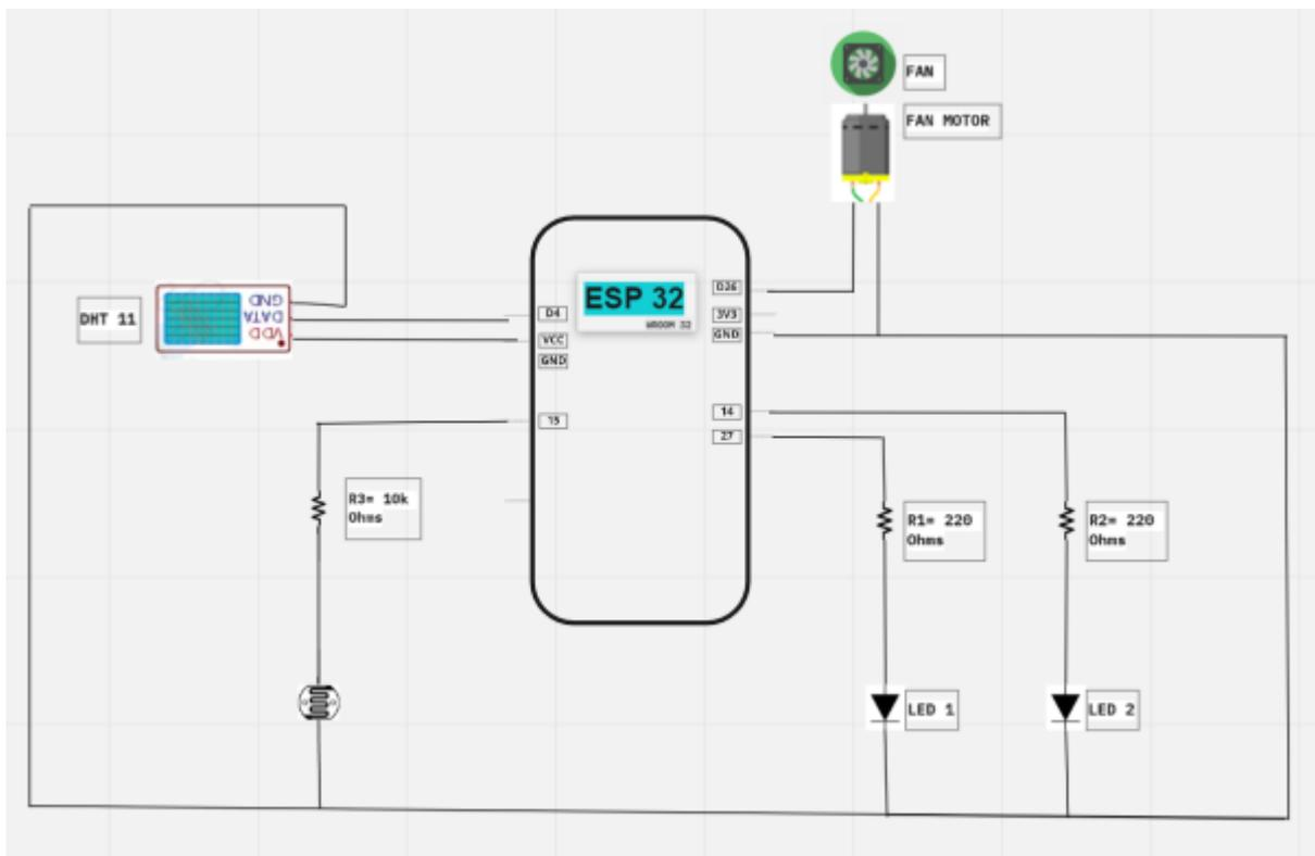
**Figure 8** Schematic Representation of the First Trial of Fan Connection to esp32.
