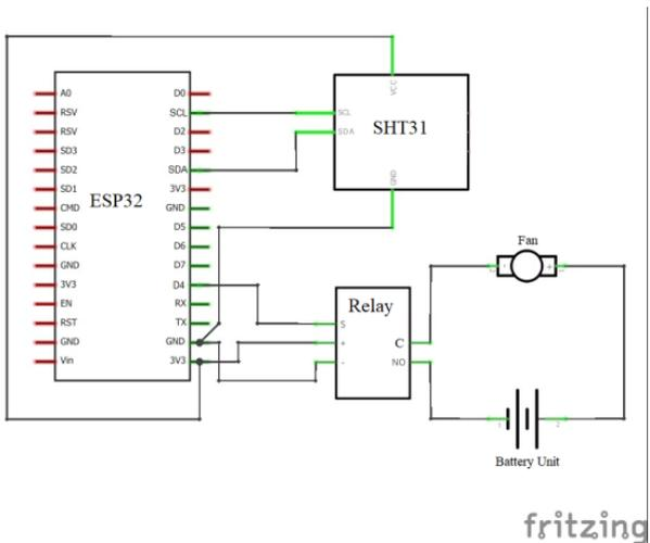
**Figure 11** - Schematics of the setup (Akuri)
