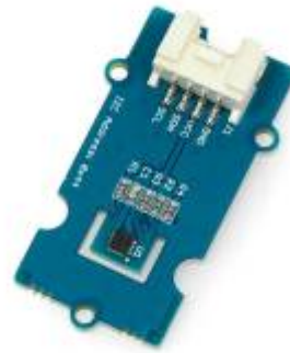
Figure 6 SHT31 Temperature and Humidity Sensor.
