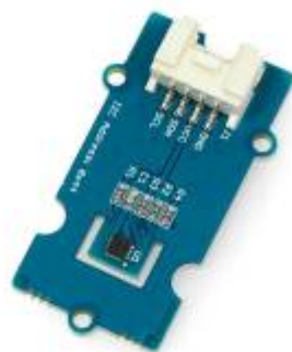
Figure 6 SHT31 Temperature and Humidity Sensor.
