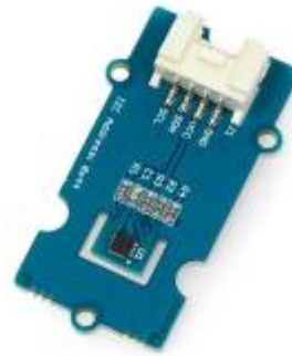
Figure 6 SHT31 Temperature and Humidity Sensor.
