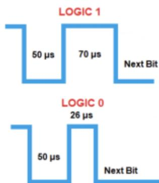
**Figure #** DHT22 Logic Signal formation. Source: <https://www.teachmemicro.com/how-dht22-sensor-works///>
