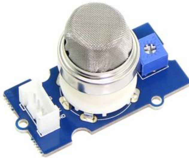
Figure 1. MQ2 Sensor. Source: https://lastminuteengineers.com/mq2-gas-senser-arduino-tutorial/
