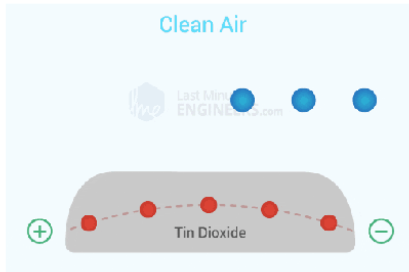
Figure 2. Chemical process altering the resistance in the module which causes a change in voltage output. Source: http://lastminuteengineers.com }}
