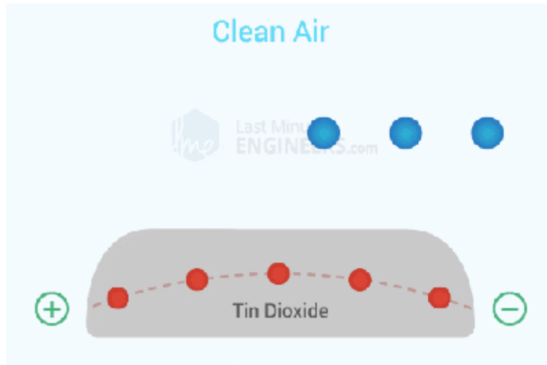
Figure 2.4 Chemical process altering the resistance in the module which causes a change in voltage output. Source: http://lastminuteengineers.com }}
