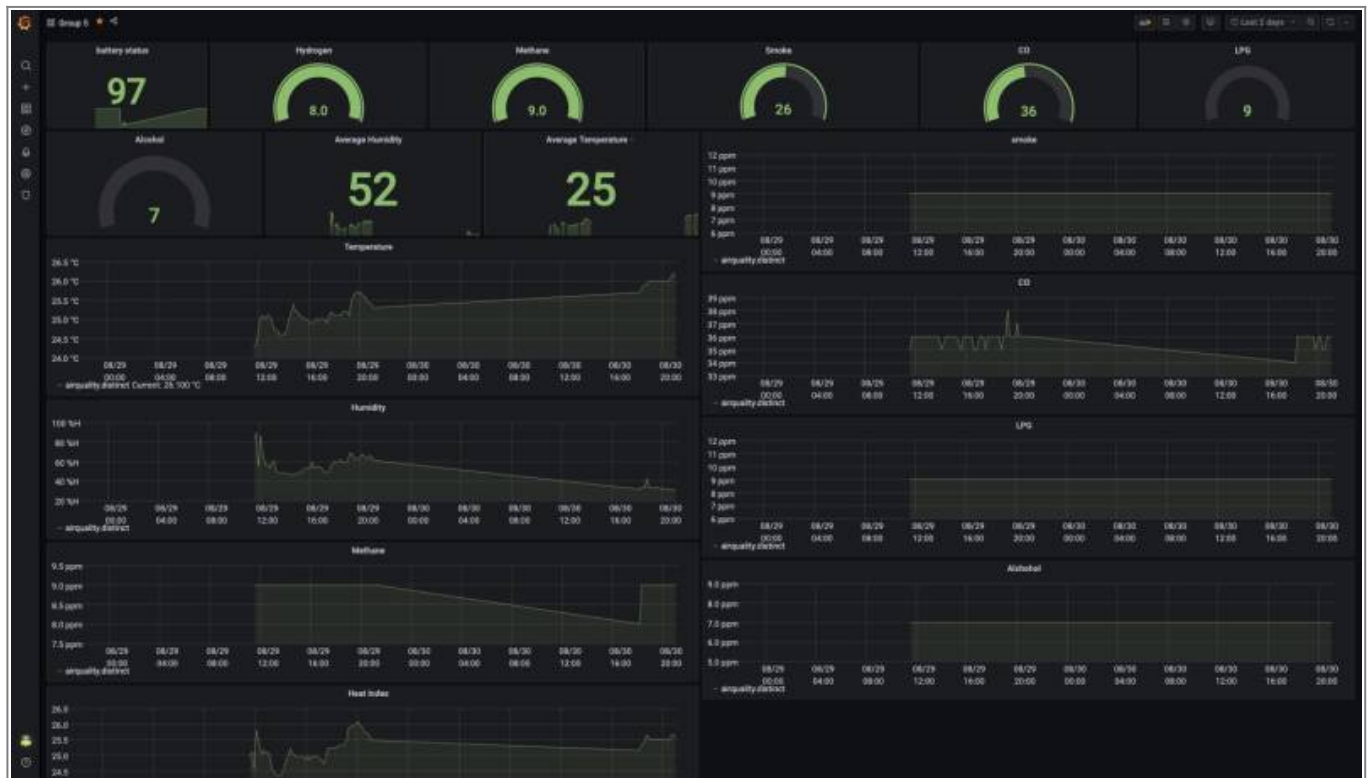
figure # Measurement result of DHT22 and MQ2 sensors visualised on grafana
