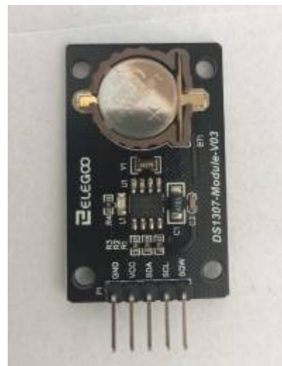
Fig. 4: RTC DS1307 Module (Taken by Emilie Streichsbier)
