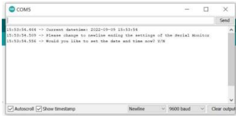
Fig. 5: Setting the time in the serial monitor
