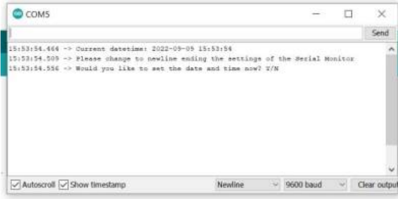
Fig. 5: Setting the time in the serial monitor
