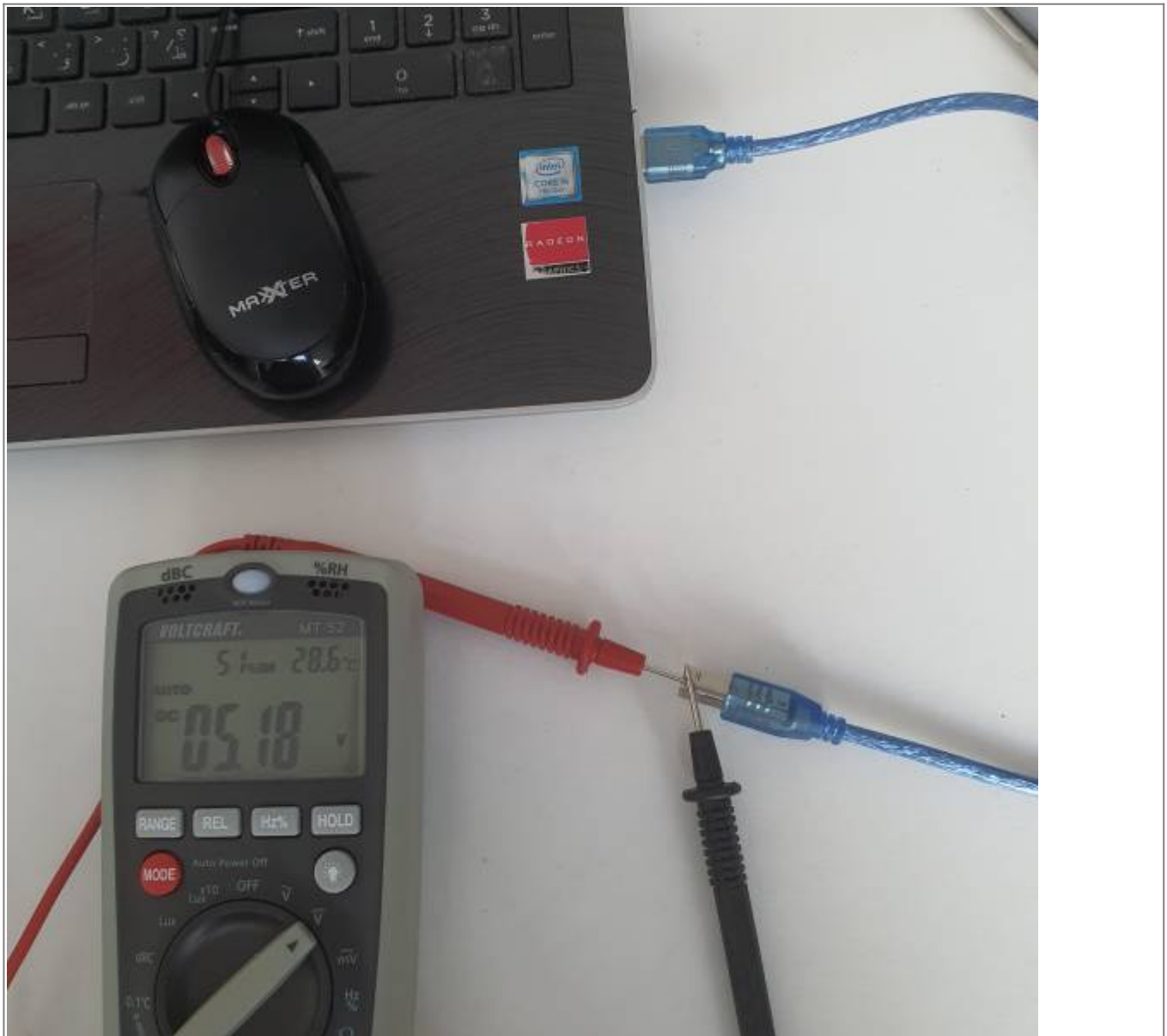
Figure 20 Measuring the voltage supplied by the Laptop USB port directly, Photo by Ziad Helou
