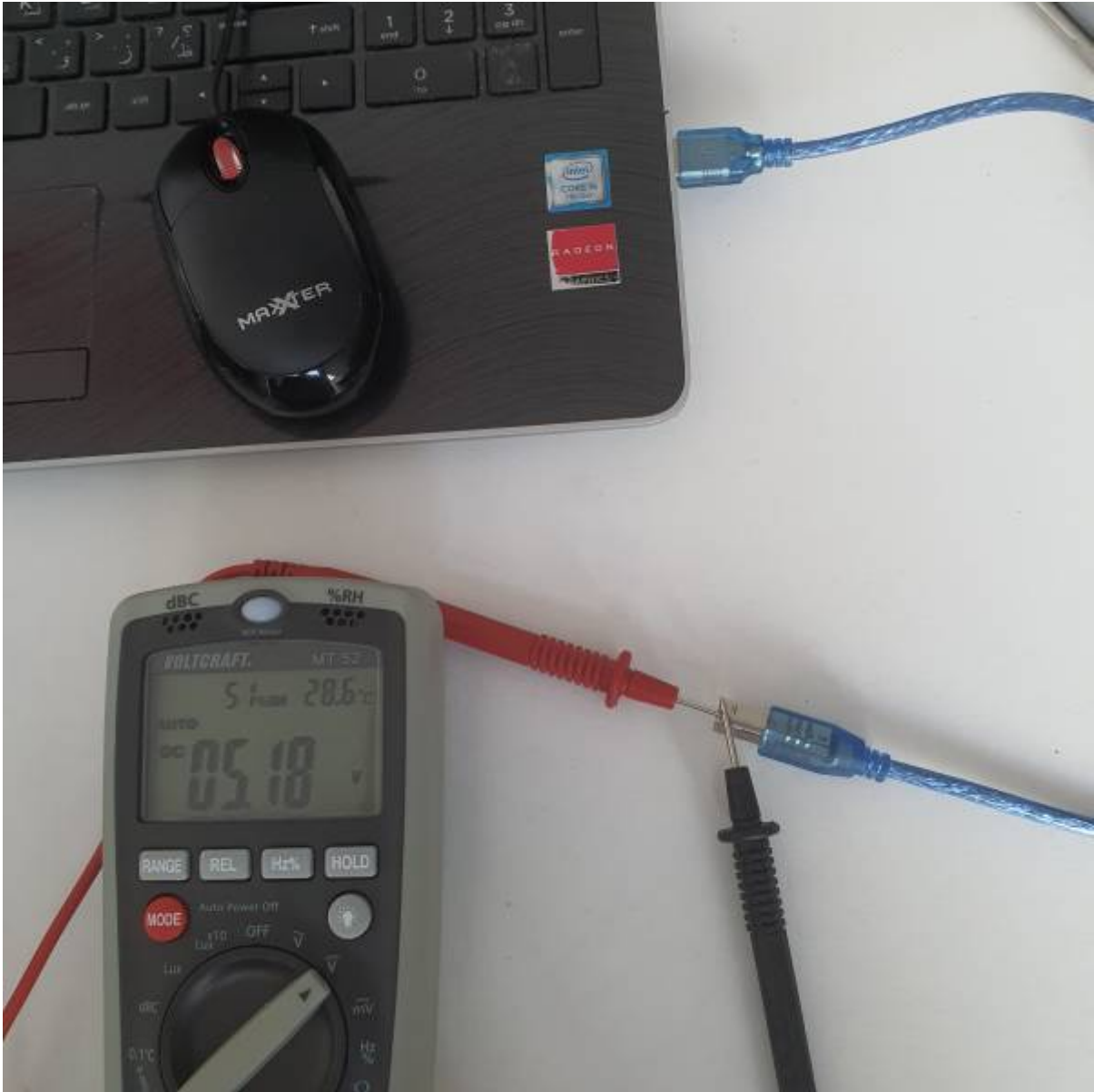
When connecting the Laptop USB port using a micro cable USB to the ESP32 and measuring the output voltage from the pins 5V and 3V3, we got the voltage required to power the sensors - almost 5 volts:
