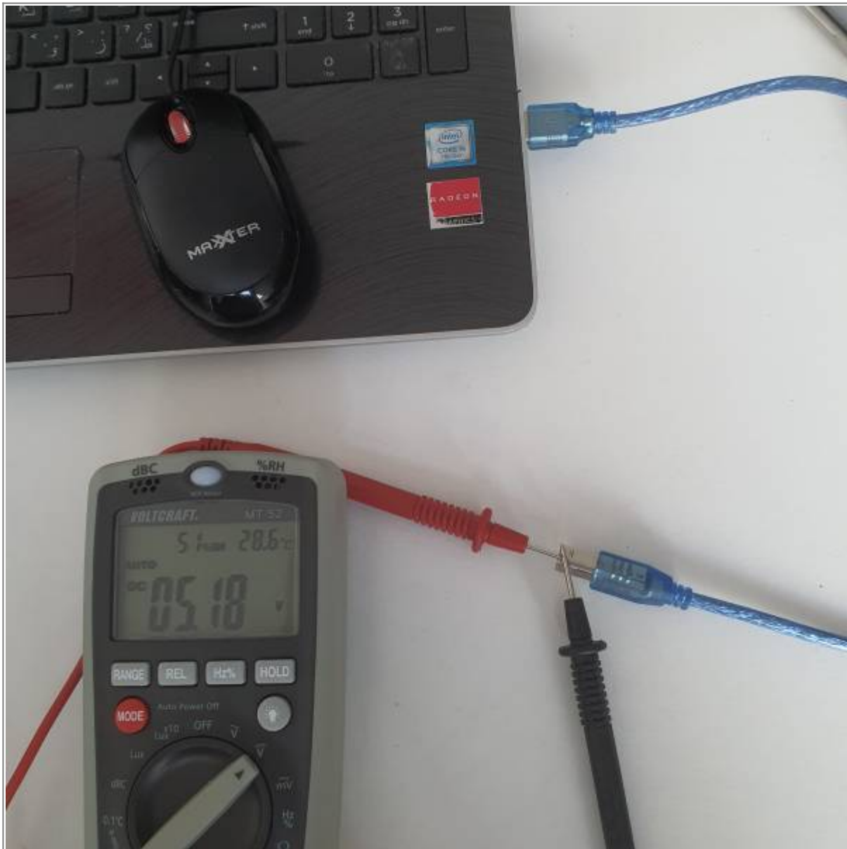
Figure 18 Measuring the voltage supplied by the Laptop USB port directly
