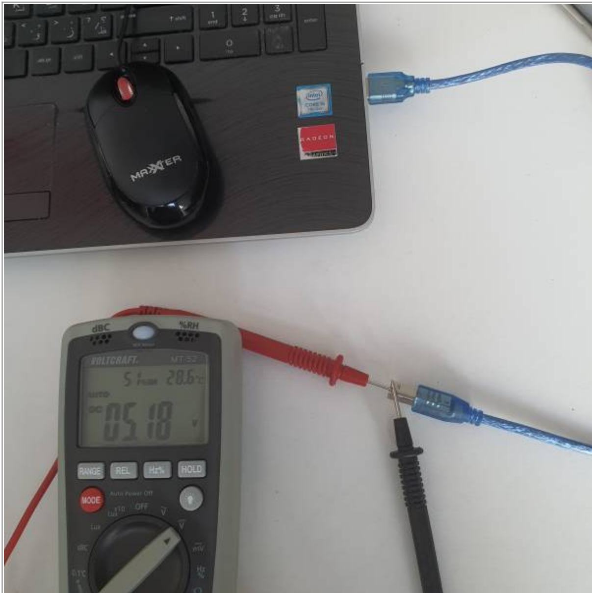
Figure 20 Measuring the voltage supplied by the Laptop USB port directly
