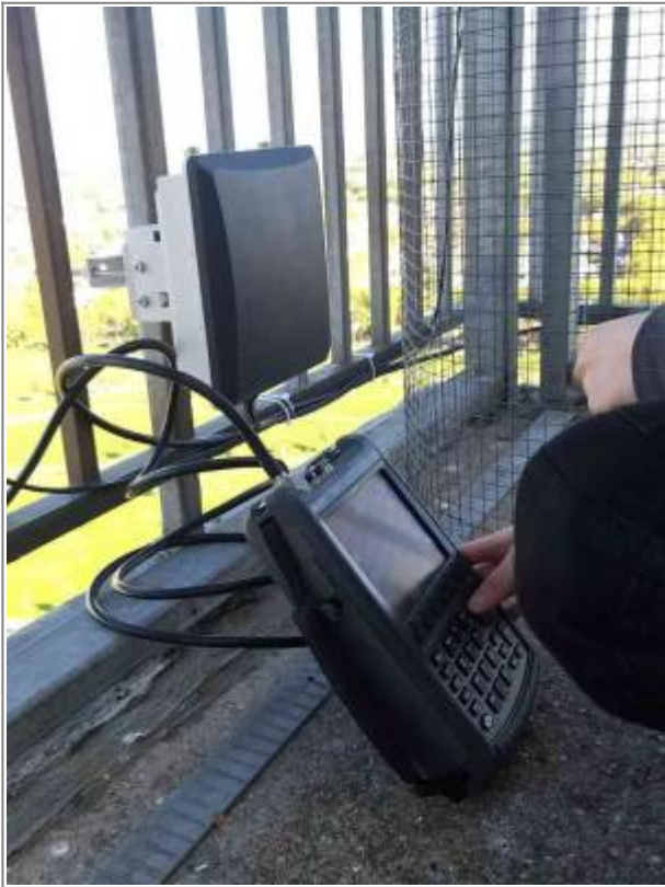
Fig.: Using a vector network analyzer to tune the antenne performance.
