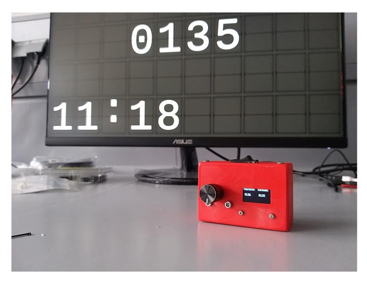
The controller consists of an ESP8266 with a battery, a rotary encoder, and a small display. All together in a 3d-printed housing. More information can be found here: Link to the Readme
