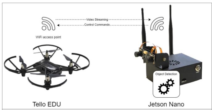
The Tello drone video stream is used as input for NVIDIA Jetson Nano object detector.
