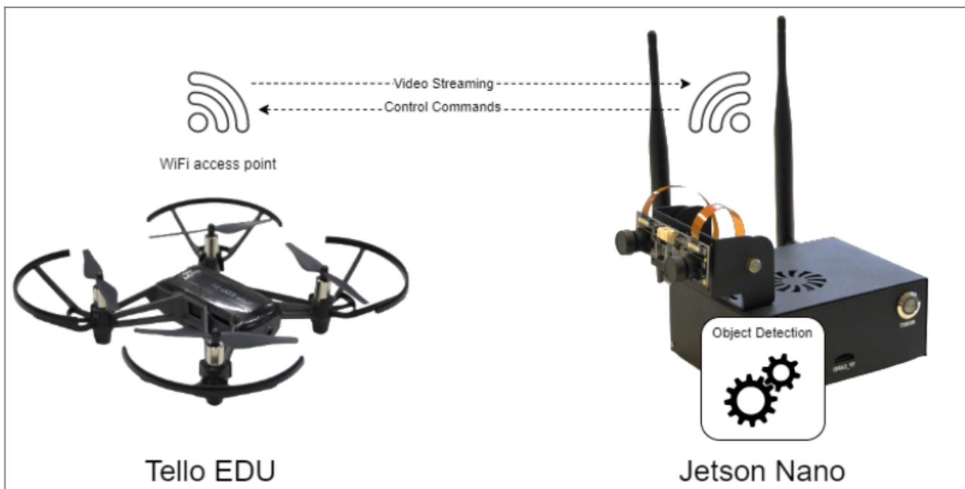
The Tello drone video stream is used as input for NVIDIA Jetson Nano object detector.
