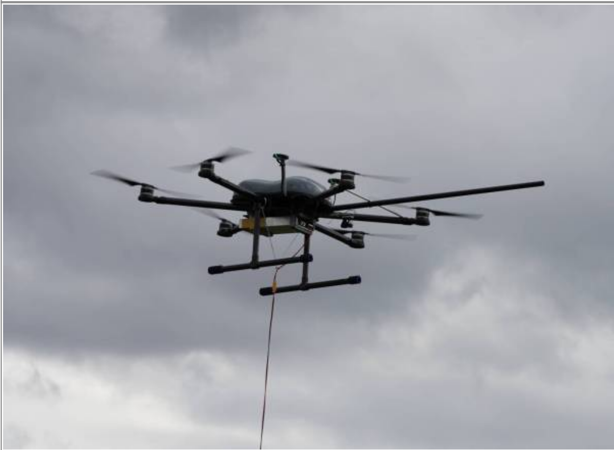
Fig.: Tethered utility drone with sprayer.
