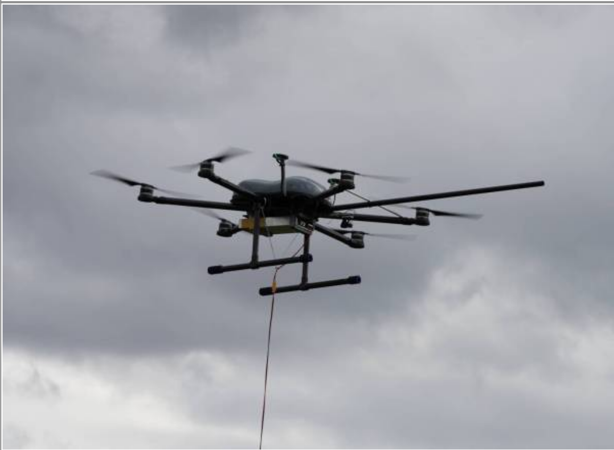
Fig.: Tethered utility drone with sprayer.
