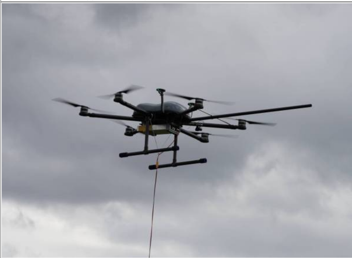
Fig.: Tethered utility drone with sprayer.
