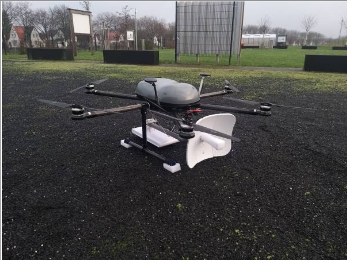
Fig.: Tethered utility drone with network devices.
