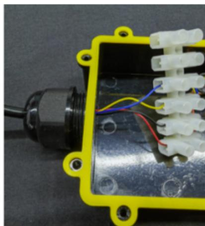
3. Connect the sensor wire to the junction box.
