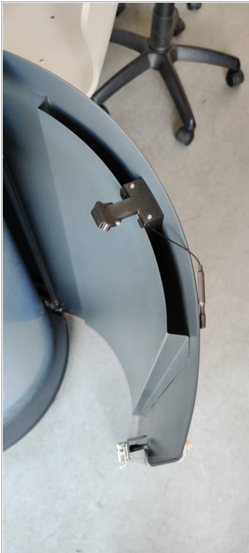
Fig.: Sensor Module installed in the door of the trashcan
