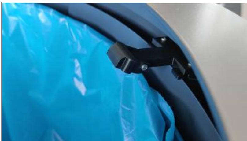
Fig.: Sensor Module installed in the door of the trashcan
