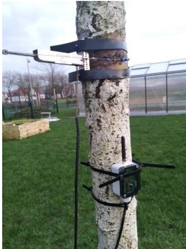
Fig. 1: Dendrometer at the Green Fab Lab using local LoraWAN (Zechenfunk)
