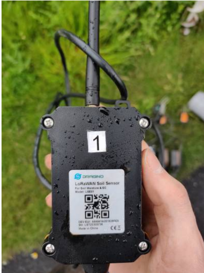
Waterproof housing of the LoRa node.
