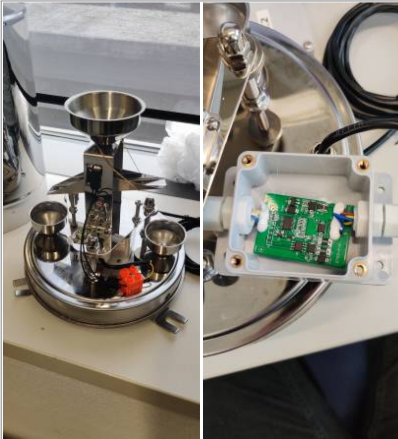
Inside of the Rain Gauge and PCB
