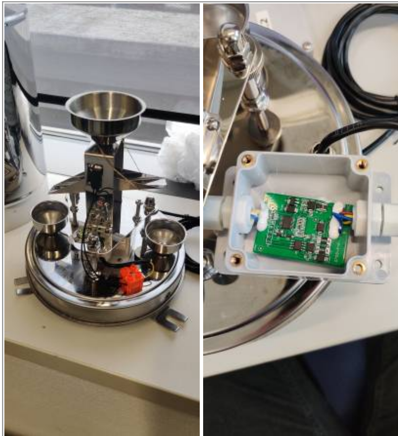
Inside of the Rain Gauge and PCB
