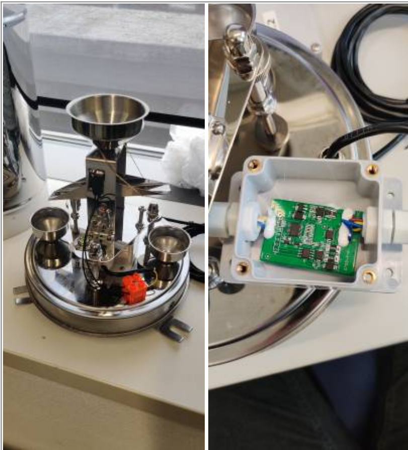
Inside of the Rain Gauge and PCB
