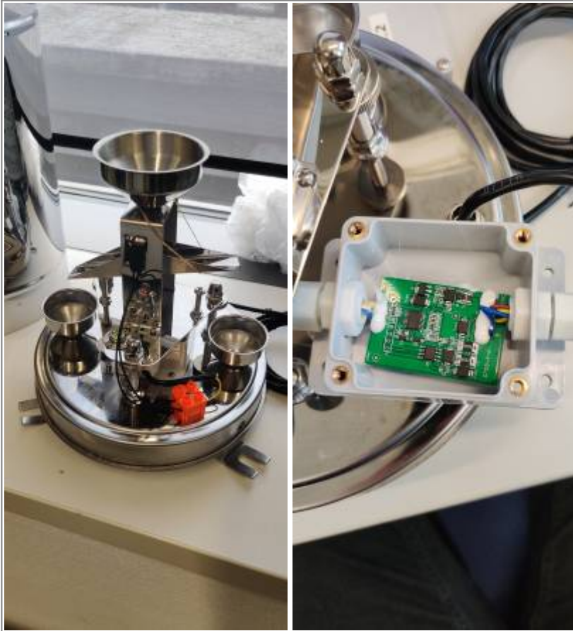
Inside of the Rain Gauge and PCB
