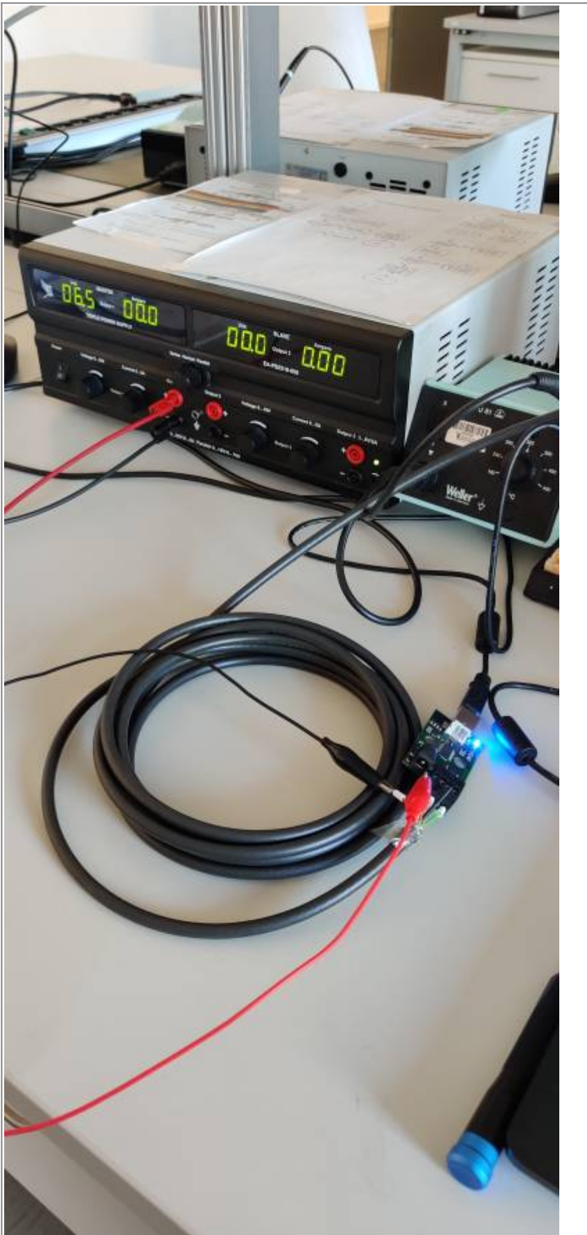
Fig.: Connecting to the WXT536 with an rs485 to USB converter
