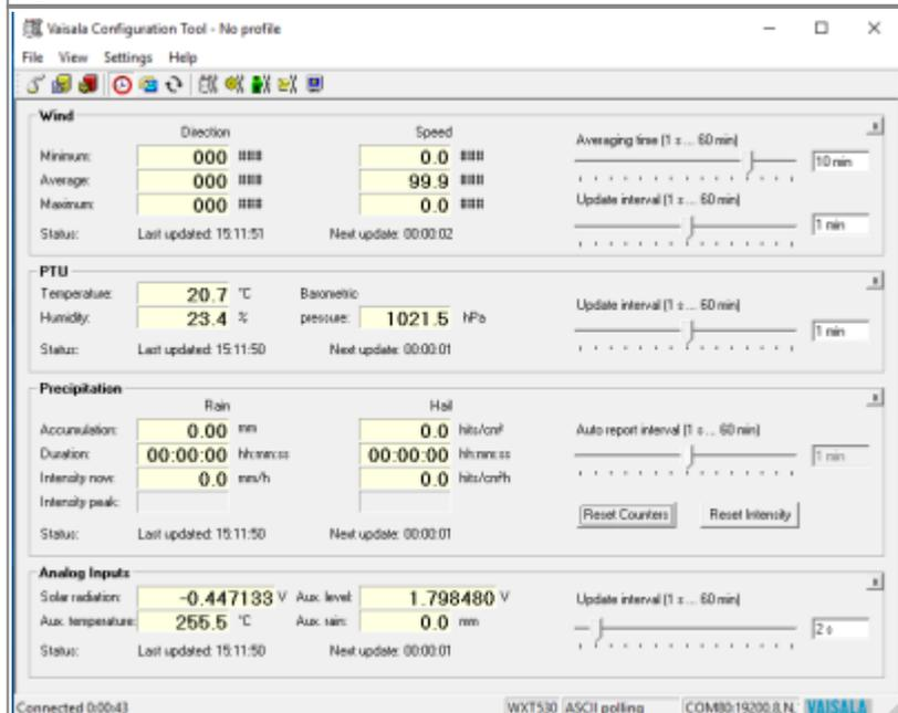
Fig.: Reading the Data with the Vaisala Configuration Tool
