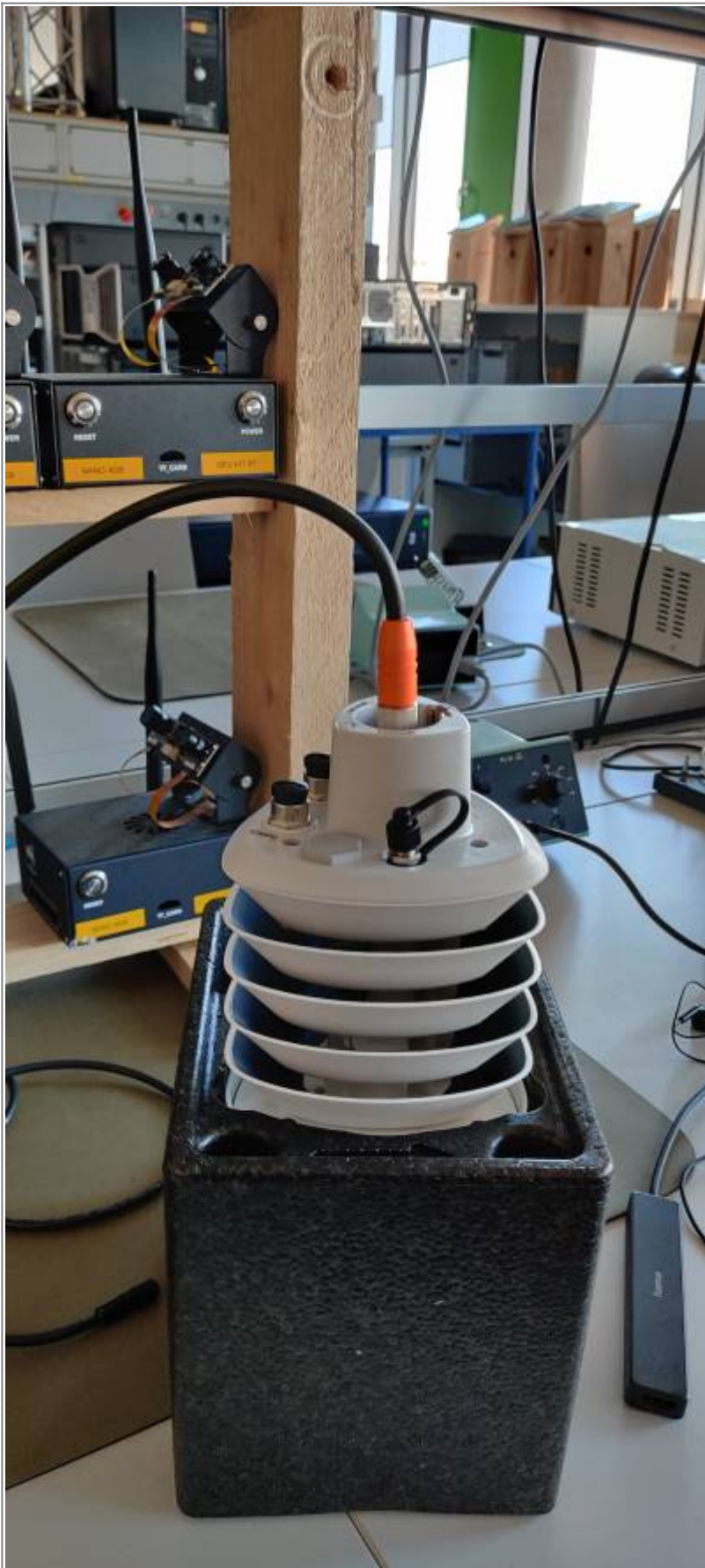
Fig.: Connecting to the WXT536 with an rs485 to USB converter
