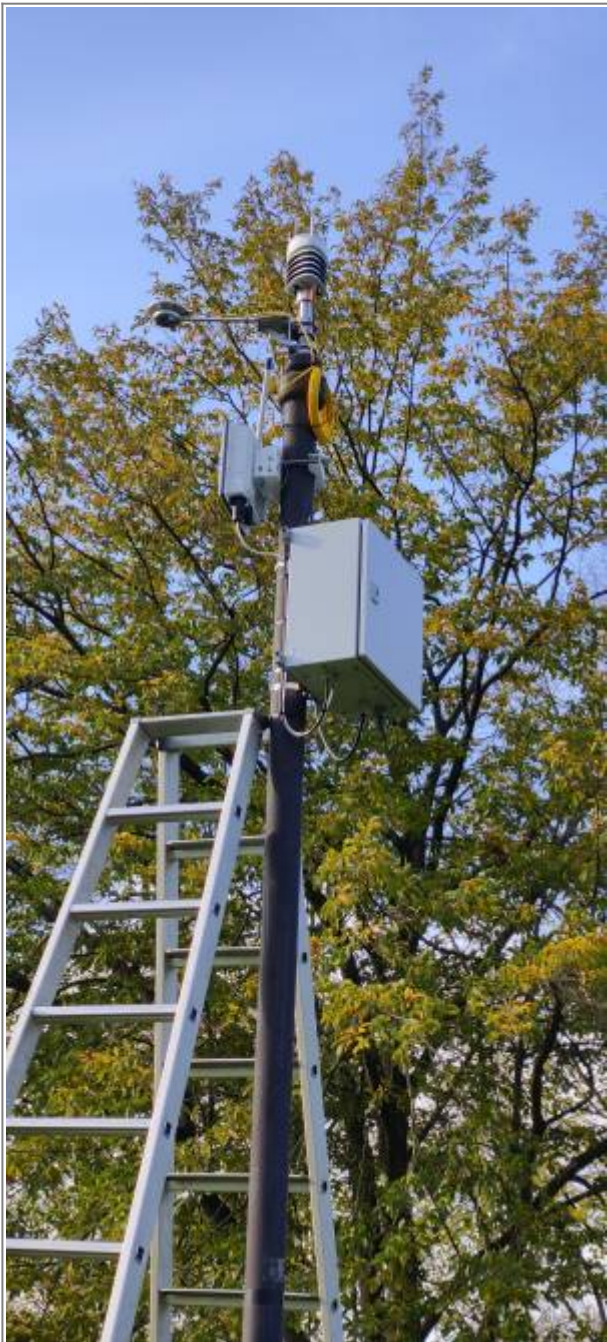
Fig.: Weather station mounted on a pole at Forstgarten in Kleve
