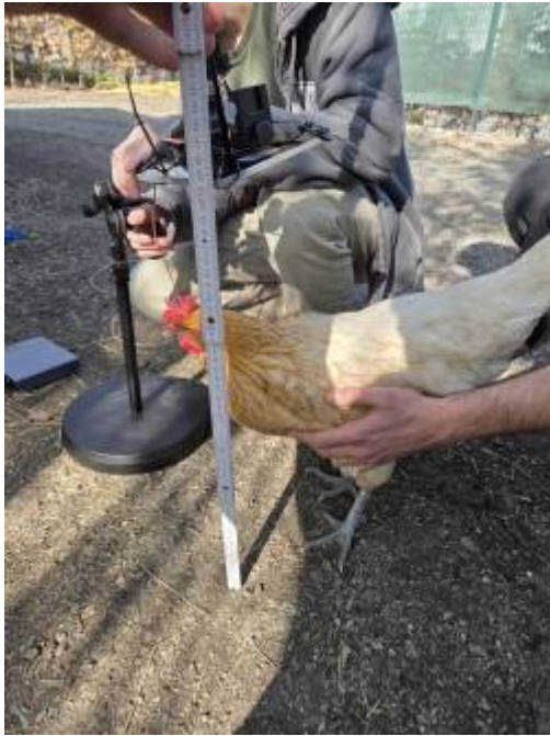
Antenna placed horizontally at 50 cm height on the ground able to read the rfid tag reliably. Antenna was then lifted up to at most 100 cm and still able to read the rfid tag (read range approximately 25-70cm).
