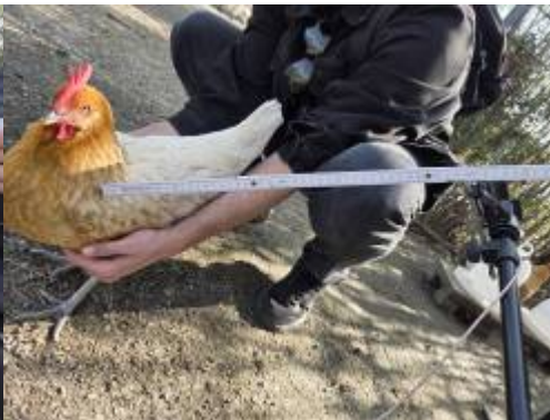
44 cm read range with antenna tested from tilted 35 to 45°
