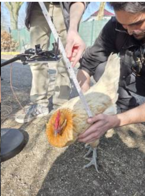
Antenna placed horizontally at 50 cm height on the ground able to read the rfid tag reliably. Antenna was then lifted up to at most 100 cm and still able to read the rfid tag (read range approximately 25-70cm).
