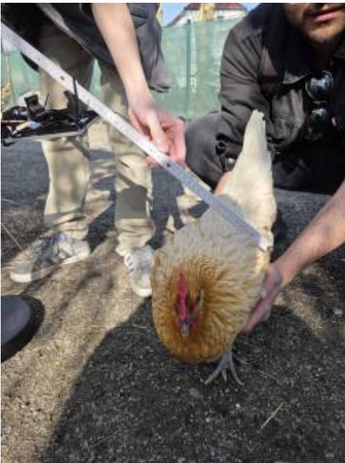
33 cm read range from the side of the antenna
