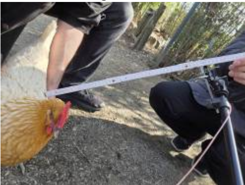
44 cm read range with antenna tested from tilted 35 to 45°
