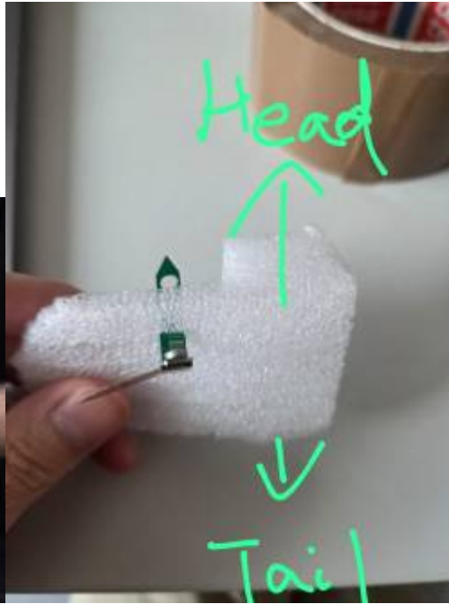
Tag is mounted from outer part of the wing to inner part as shown on the right. The rfid tag is faced outside
