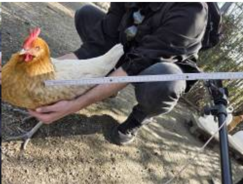
44 cm read range with antenna tested from tilted 35 to 45°
